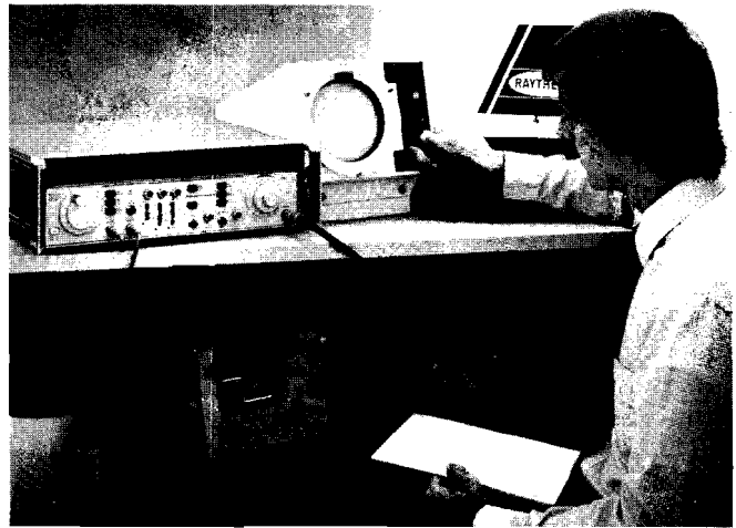
Option 001 for the HP 8683/84D generators provides 10 mW output power in the frequency-doubled band, as well as in the standard band.
