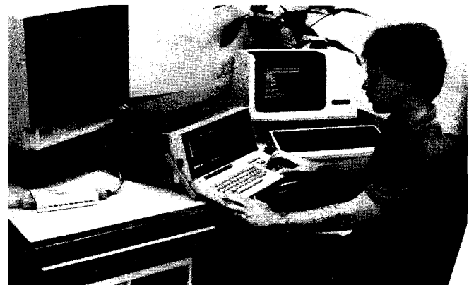
An advanced data communications analyzer, the HP 4953A Protocol Analyzer, allows the user to download test programs to data-terminal equipment to analyze data communications. The HP 4953A can also verify system performance and troubleshoot problems in your network.
